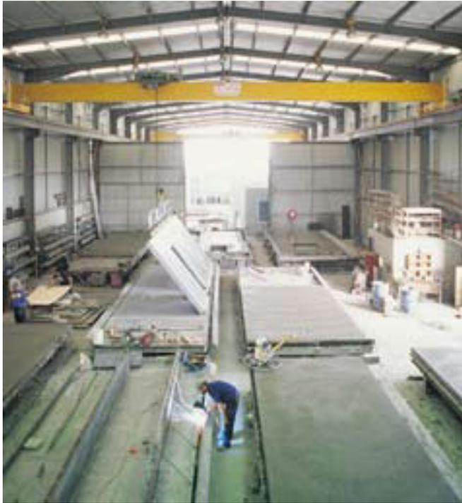
*LEFT: Precast concrete is manufactured in a controlled environment allowing more efficient use of materials with very little waste.*
