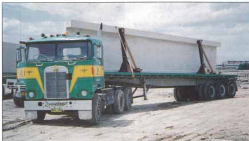
FIRM ACCESS AND EGRESS WITH ADEQUATE TURNING SPACE FOR CRANE AND DELIVERY VEHICLE IS VITAL.
