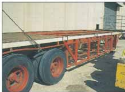
PURPOSE-DESIGNED TRAILER FOR TRANSPORTING LARGE (DEEP) PANELS. NOTE THE SUPPORTING FRAMEWORK BELOW TRAY LEVEL.
