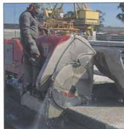
PANELS BEING SAWN TO CLIENT'S REQUIRED LENGTH
