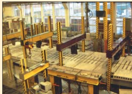
Figure 8: Hollowcore slabs with opened cores
