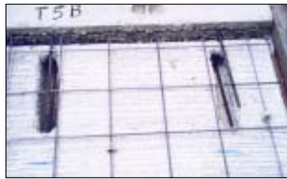
Test setup for a 1200 wide floor plank with the top flange removed from 2 cores. Two pairs of 2 off N12 reinforcing bars are screwed into ferrules cast into the wall panel. A RF72 mesh is positioned on top of the planks and a 70 mm structural concrete topping is placed that encases the N12 bars and provides a flat floor.
