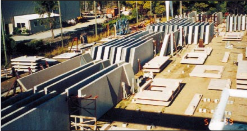
Panels in storage at precaster's yard awaiting delivery (above) and a 6.2 m x 3 m precast panel being transported from factory (left)
