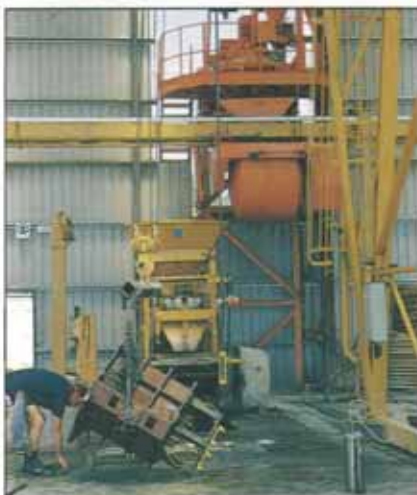
TYPICAL WORK STATION – MIXER DISCHARGES INTO HOPPER, CONCRETE IS THEN CONVEYED TO POINT OF CASTING ON A MOVING BELT.
