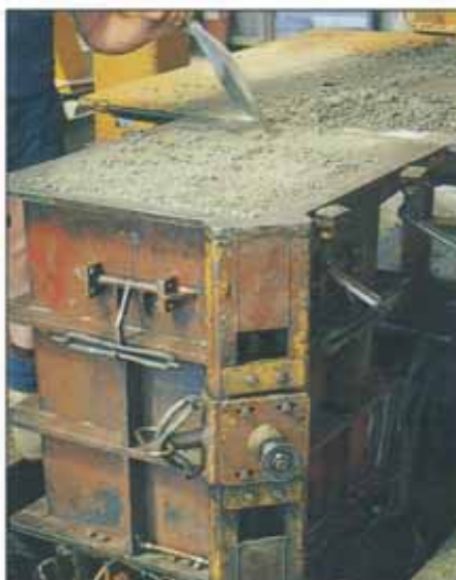
TYPICAL WORK STATION – MIXER DISCHARGES INTO HOPPER, CONCRETE IS THEN CONVEYED TO POINT OF CASTING ON A MOVING BELT.
