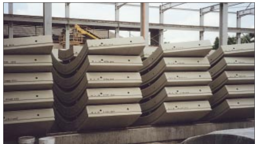
COATED SEGMENTS READY FOR DELIVERY TO SITE
