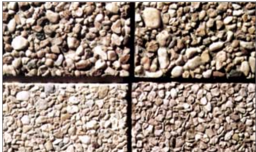
PHOTOGRAPH 7 VARIOUS APPEARANCES OF EXPOSURE. THIS RANGE CAN BE FURTHER EXTENDED USING DIFFERENT SIZED AGGREGATES.
