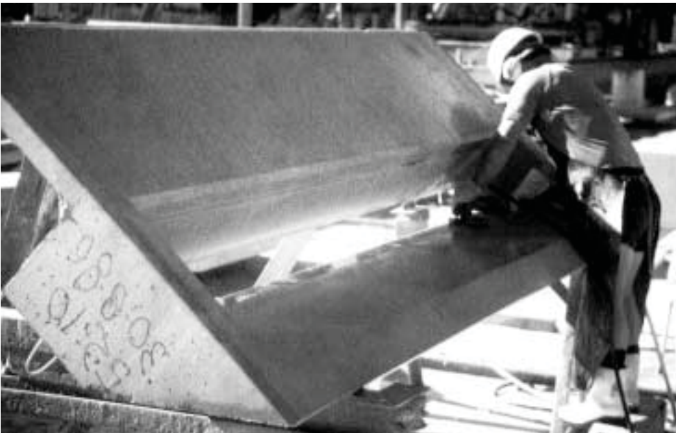
Facing page – State Parliament Offices, Sydney, where yellow-brown quartzite aggregate was exposed by honing and acid-etching; top – panel shape requiring some costly hand-finishing; bottom – finish of precast panels, State Parliament Offices, Sydney
