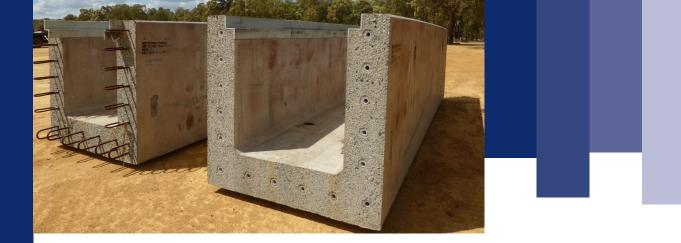
the trench culverts to be produced off site. The precast solution will see the trenches manufactured in PERMAcast's ISO 9001 Quality controlled factory environment.
